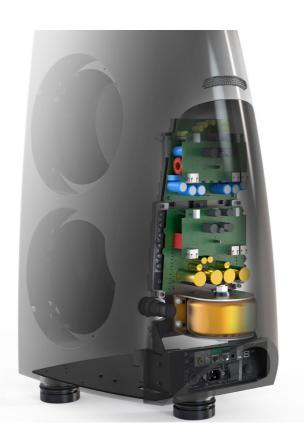
The DAC boards are mounted directly above the two amplifier boards This reduces the length of the analogue audio paths which minimises interference on the analogue signals. Each DAC board receives its own power from ultra-low noise linear regulators which greatly improves the electrical isolation between the digital and analogue sections.
